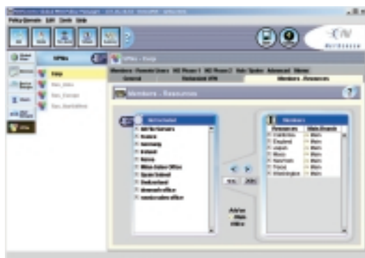
The point and click interface allows new resources to be added to a VPN in minutes.
