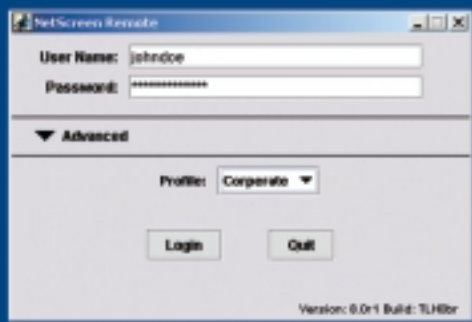
NetScreen-Remote VPN Client authenticates the user prior to retrieving VPN Policies
