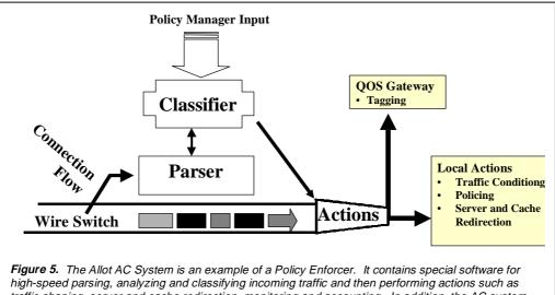
high-speed parsing, analyzing and classifying incoming traffic and then performing actions such as traffic shaping, server and cache redirection, monitoring and accounting. In addition, the AC system has the ability to perform QoS gateway functionality whereby it can translate and tag traffic according to standards-based signaling protocols such as Differentiated Services, RSVP and MPLS.
